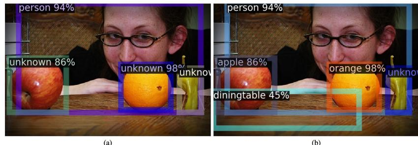
Detections on the left are produced by our method after learning a set of few classes which does not include edibles. We are able to identify them and correctly labels them as *unknown*. When the model is eventually taught to detect fruits, these instances are labelled correctly as in (b); without forgetting to detect *person*. An unidentified class instance still remains, and is successfully labelled *unknown*.
